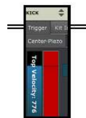
Pic 14: Trigger Input Overload
