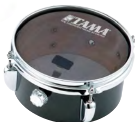
TMP8S This snare pad is an actual 4" x 8" inch drum with a mesh head. It has a half cut snare wire facing the backside of the mesh head from inside the drum. The knurled knob on the side of the shell lets you adjust the snare tension from tight to loose and off. You can also adjust the tension of the mesh as on a conventional drum.
